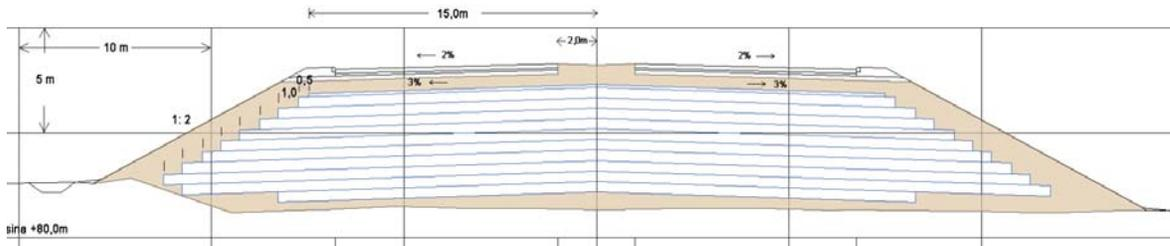
Figure 2 – Cross-section profile of designed light-weight structure with EPS-blocks at the chainage km: 187+050 of „Batajnica“ interchange basic alignment
