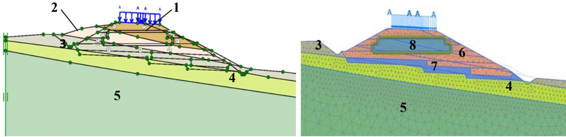
Figure 6. – Embankment model for stability back analysis on the left, and model for forecaste behaviour of new embankment by EPS geofoam blocks utilization on the right, by FEM analysis
