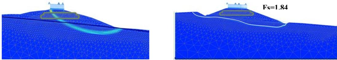
Figure 7. Global stability of old embankment, on the left, and stability of new embankment after rehabilitation measures by EPS blocks, on the right
