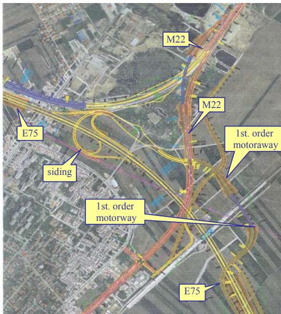
Figure 1: Aerial photo of „Batajnica“ interchange with all road routes and marked light-weight structures made of EPS-blocks
