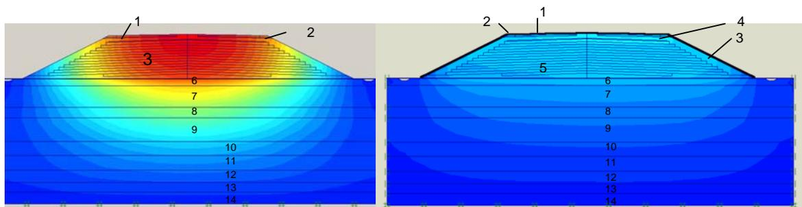
Figure 3 –Resulting vertical deformation, under road structure's own weight obtained by *PLAXIS*- model analysis of typical cross-section at km 188+450 at the interchange Batajnica basic alignment, with the
