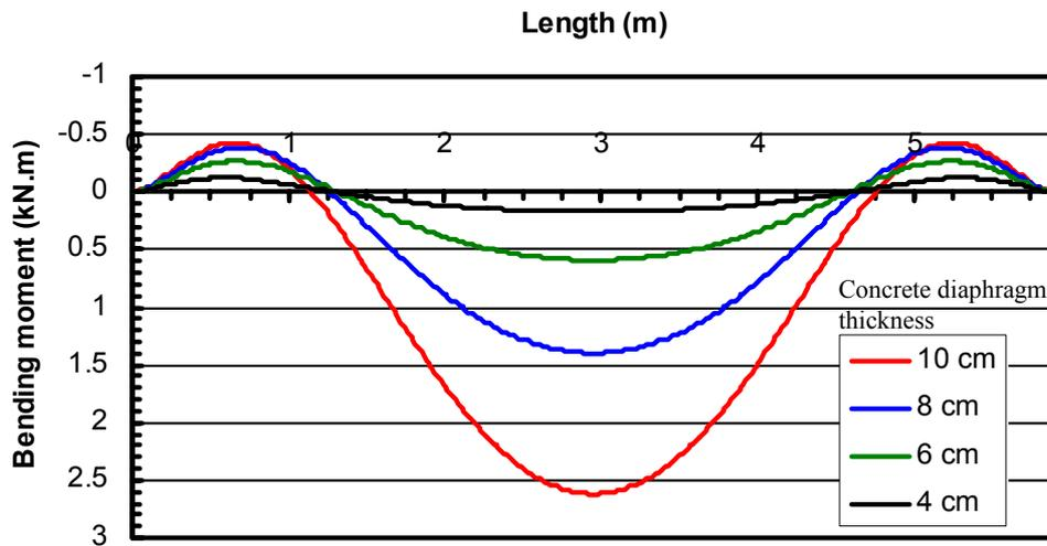
Figure 6: Induced bending moment in diaphragms of different thicknesses
