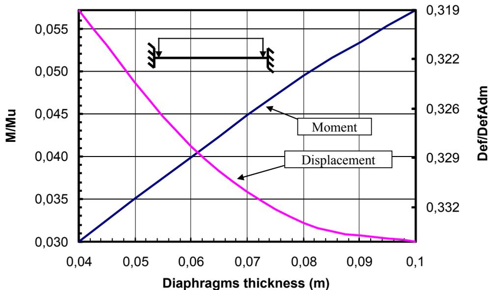
Figure 7: Relative bending moment and displacement of different diaphragms thicknesses
