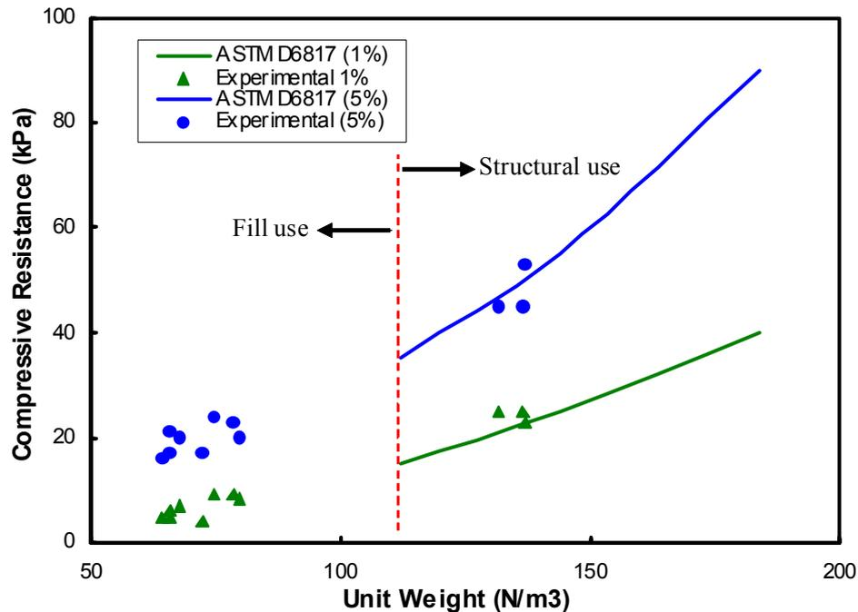
Figure 3: Relationship between compressive strength and unit weight for EPS
