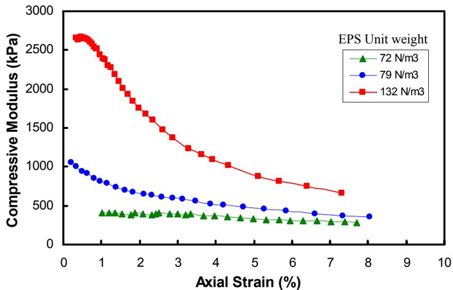
Figure 5: Compressive modulus–strain relationship
