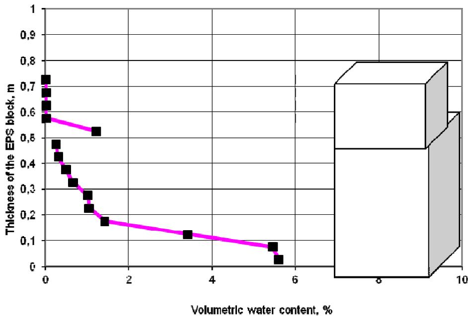
Figure 5. The volumetric water contents of EPS blocks on cross section 1197 to Turku [3].
