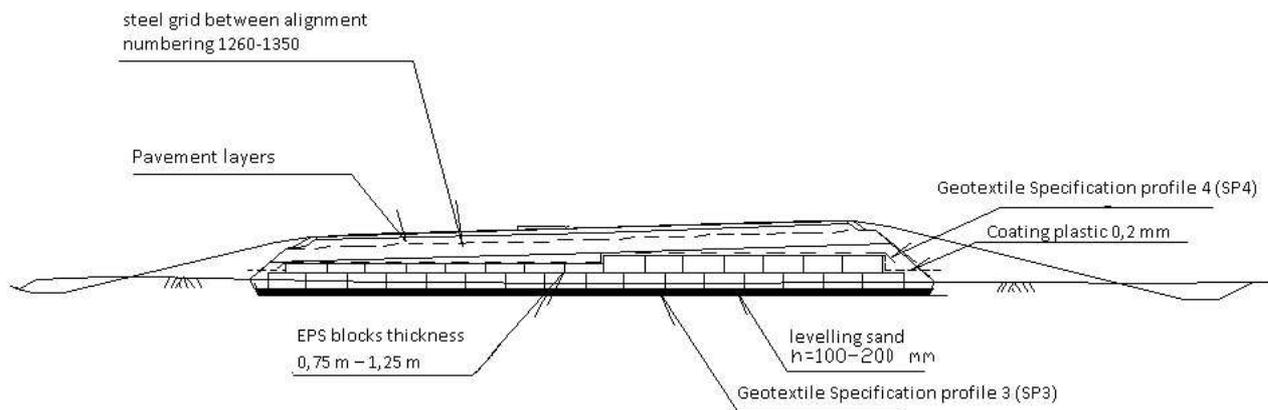
Figure 2. The cross section of the EPS embankment [2].
