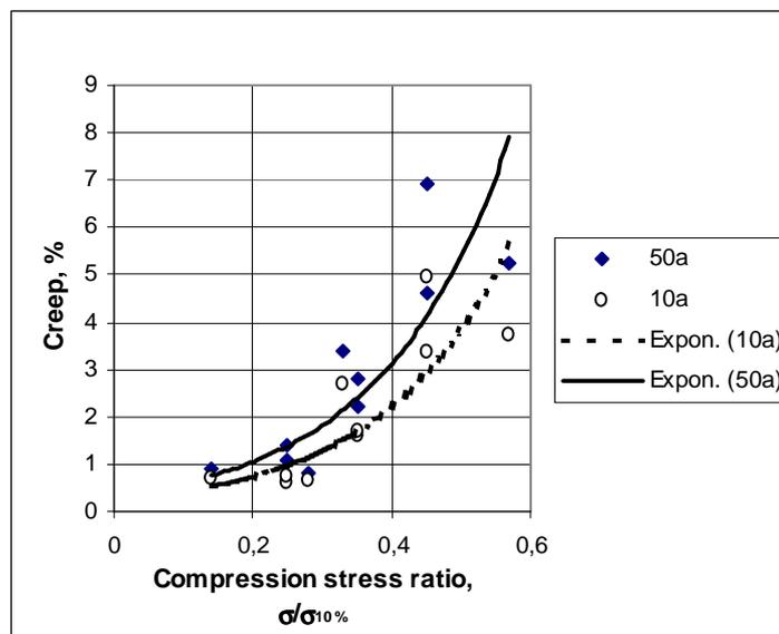
Kuva 3. Compression creep in 10 a’ 50 years vs. compression stress ratio. (10a – 10 years; 50a – 50 years)
