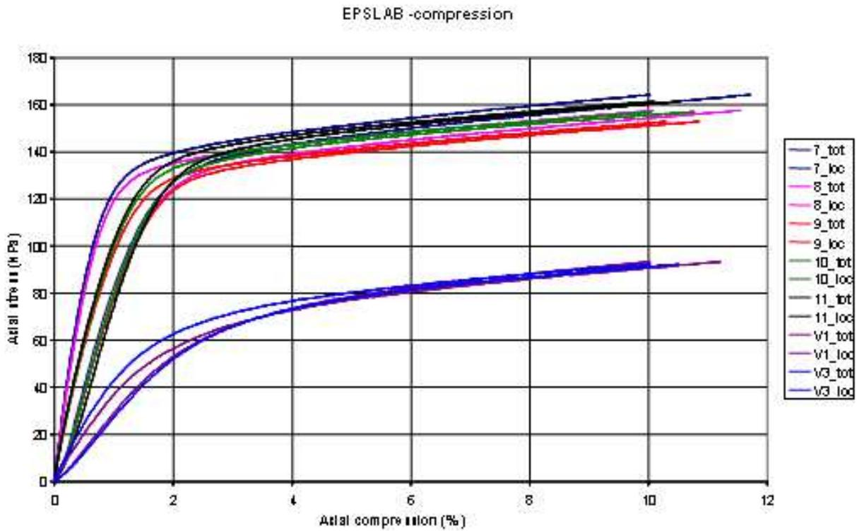
Fig 2 Compression curves of tested EPS materials. Upper set of curves: new EPS; lower sets of curves: old EPS from Pesurinkatu site. Marking of curves: “7 tot/loc” – specimen 7, compression measured between ends (tot)/between inner third points (loc).
