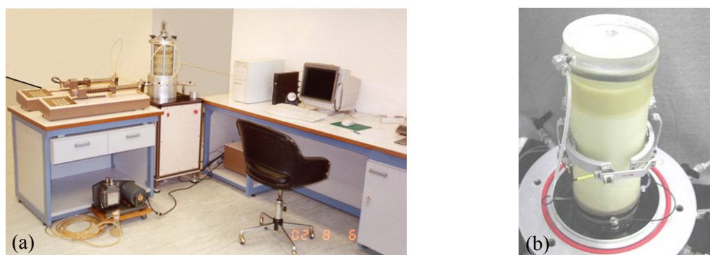
Figure 1. (a) The triaxial (cyclic/monotonic) loading system used in the laboratory program, (b) the local strain measuring transducers used in the triaxial tests on EPS specimens
