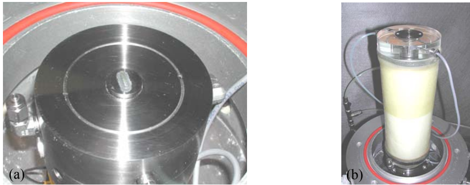
Figure 3. The bender/extender element system used in the laboratory program (a) the pedestal of the device with the insert element, (b) EPS specimen mounted in the testing system
