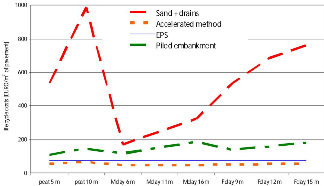
Figure 6 : Life cycle cost for different construction methods, local road GL+0.4 m, time available = 24 months.
