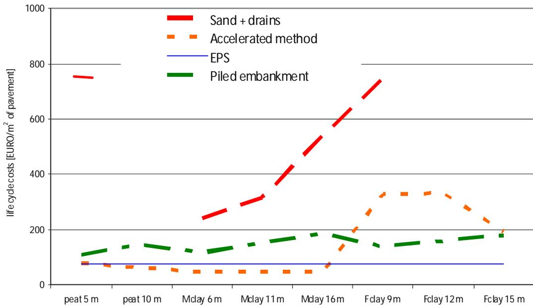
Figure 5 : Life cycle cost for different construction methods, local road GL+0.4 m, time available = 6 months.
