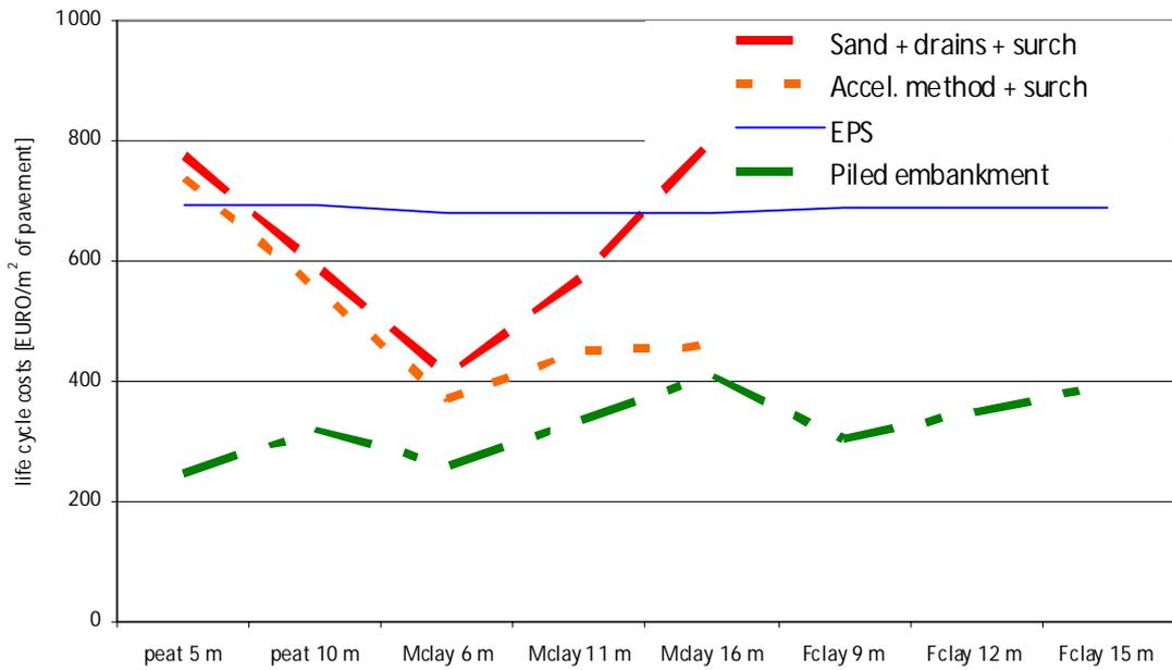
Figure 7 : Life cycle cost for different construction methods, highway GL+7.0 m, time available = 6 months.
