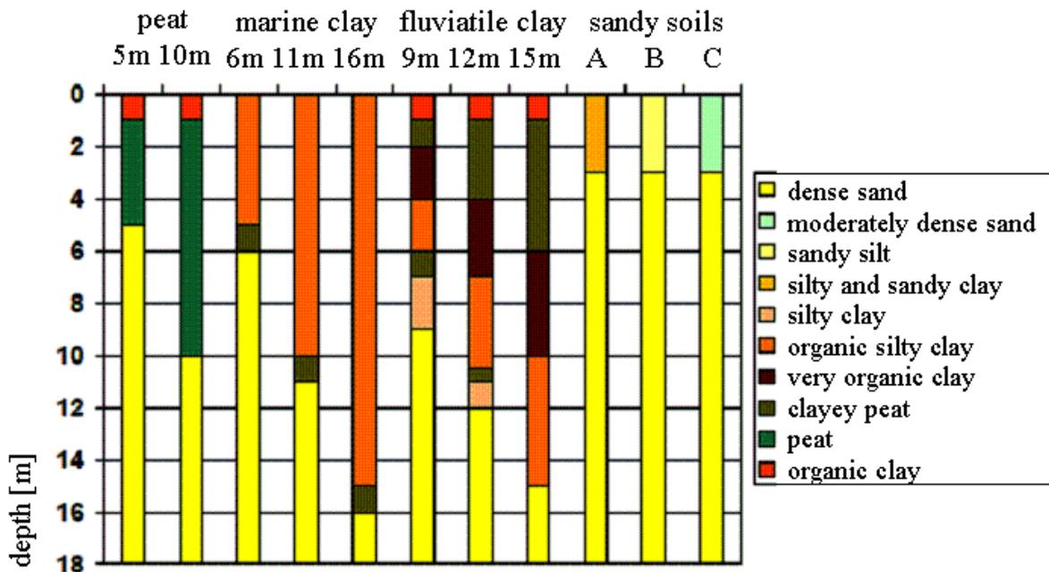
Figure 3 : Soil profiles used in this study.
