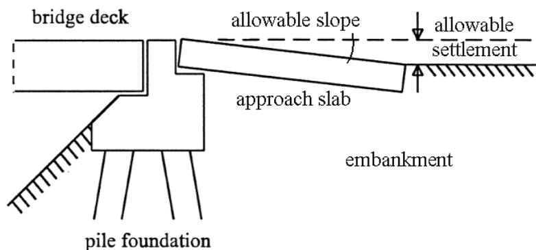
Figure 4 : Relation between allowable slope, length of approach slab and allowable settlement.
