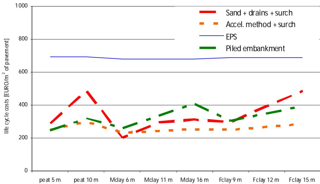
Figure 8 : Life cycle cost for different construction methods, highway GL+7.0 m, time available = 24 months.
