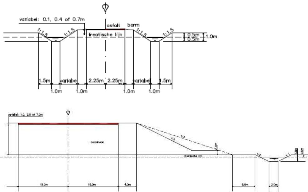
Figure 2 : Cross sections of a local road at GL+0.4 m (top) and a highway at GL+7.0 m (bottom).
