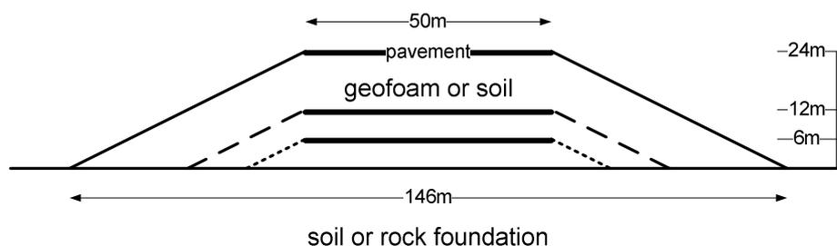
**Figure 1:** Geofabric or soil embankment sections
