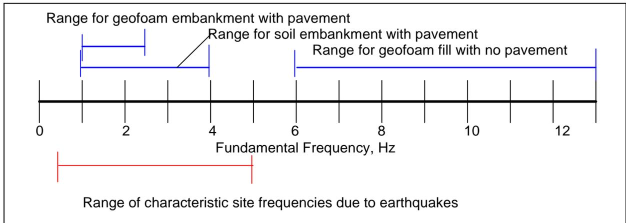
**Figure 2:** Fundamental frequency ranges for geofoam and soil embankments.
