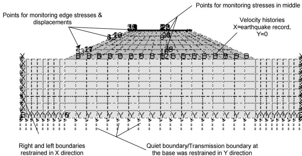
**Figure 3:** FLAC Embankment Model
