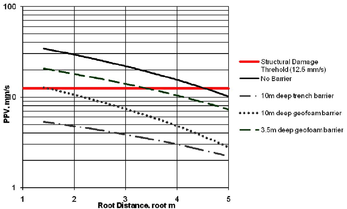
Figure 2: PPV attenuation below threshold damage limit
