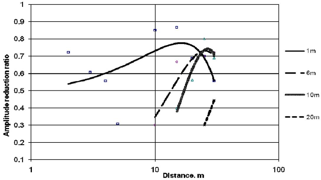
**Figure 4:** Effect of distance of wave barrier from source on vibration attenuation
