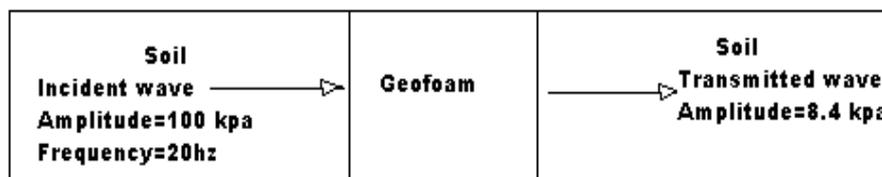
**Figure 1:** One dimensional wave transmission through geofoam
