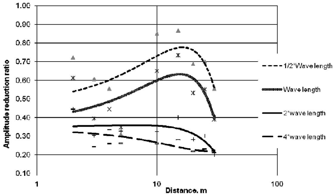
**Figure 3:** Effect of depth barrier from source on vibration attenuation
