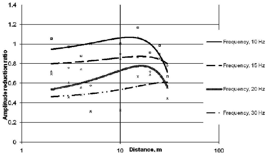
**Figure 5:** Sensitivity of amplitude reduction to the frequency of vibration
