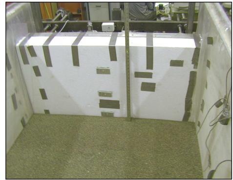
a) shaking table model with EPS geofoam buffer
