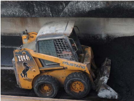
Figure 6: Cold asphalt gathered from the bottom and edges of the loading room must not be loaded onto the truck. (Photo: Bjørn Hoven)
