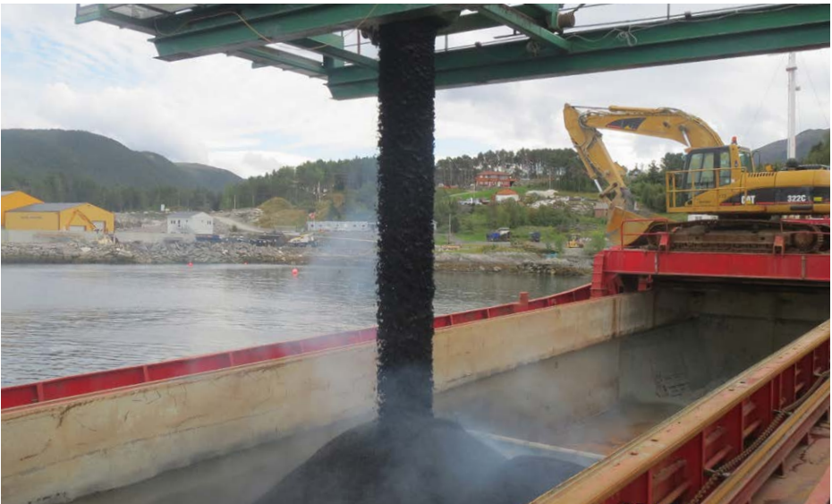
Figure 1: High falling distance results in cooling and segregation. (Photo: Bjørn Hoven)
