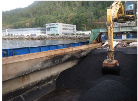
Figure 6: Cold asphalt gathered from the bottom and edges of the loading room must not be loaded onto the truck. (Photo: Bjørn Hoven)
