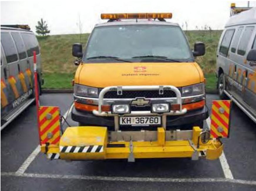
**Figure 6: Ultra-sound based pavement monitoring system**
