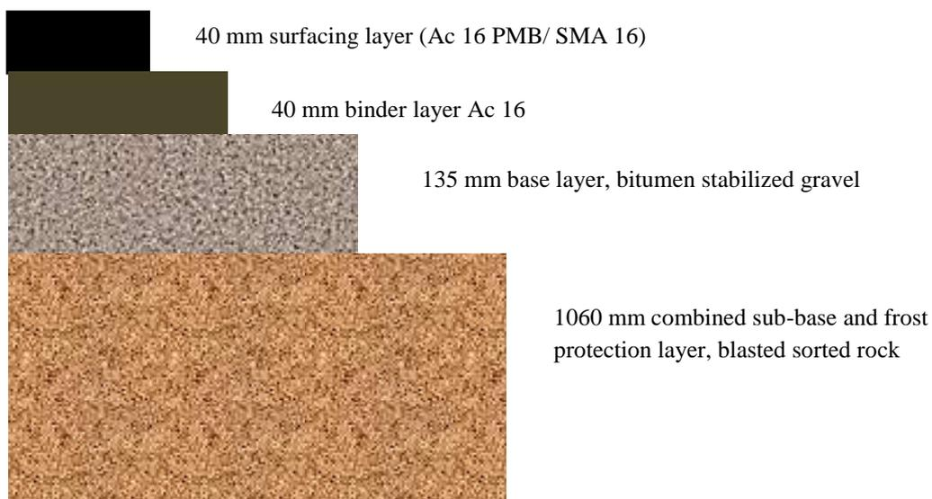
**Figure 1: Pavement structure for the test sections**
