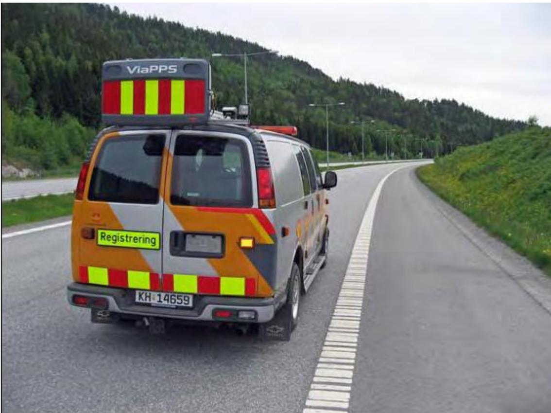
**Figure 7: Pavement profile scanner (Via PPS)**
