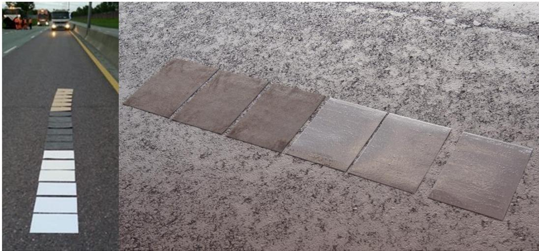
Figure 1: Trials for measurement of tack coat application rates
