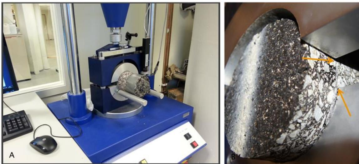
Figure 2: Shear bond strength test equipment and specimen.
