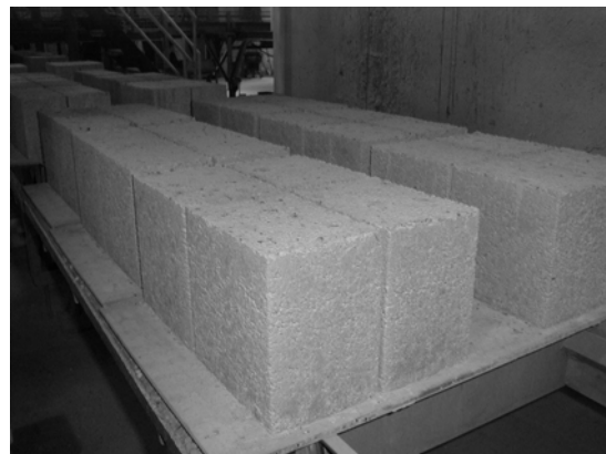
Figure 5 Building blocks with 30 % recycled aggregates (0-4 mm) (Picture: Bente Lillestøl, Veidekke ASA)
