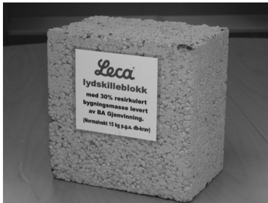
Figure 5 Building blocks with 30 % recycled aggregates (0-4 mm) (Picture: Bente Lillestøl, Veidekke ASA)
