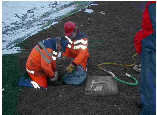
Figure 8 Sampling of compacted material
