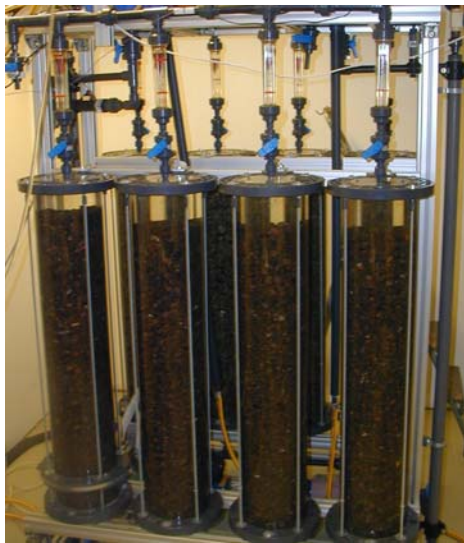
Figure 4: Test set-up for chemical deterioration of recycled aggregate
