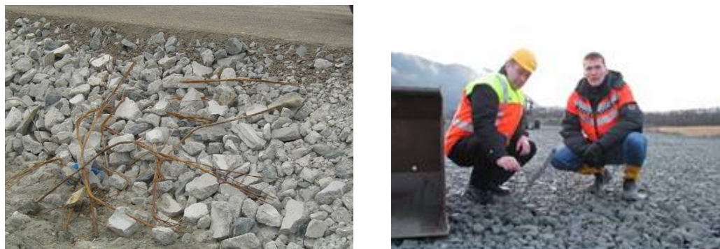
Figure 8: Remaining steel bars may cause a lot of trouble
