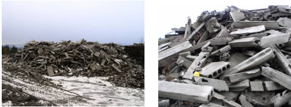
Figure 3: Element concrete stockpile
