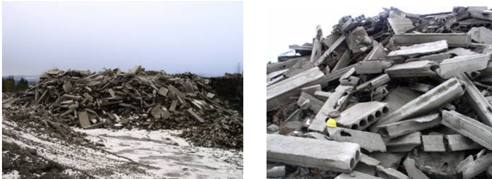
Figure 3. Element concrete stockpile
