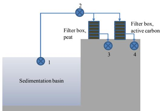
Figure 1. Outline of the experimental setup. Arrows indicate the water flow through the experiment. Crossed circles represent the various water sampling locations: 1 = pre sedimentation during the tunnel wash, 2 = after sedimentation, 3 and 4 = after filter treatment unit (FTU) filled with peat and activated carbon, respectively.
