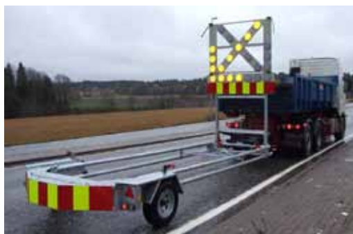
Figure 4.12 Energy absorbing equipment on vehicles (examples).
