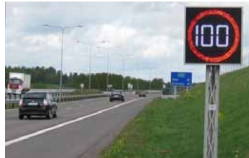
Figure 2.2: Example of a light-emitting up matrix sign.
