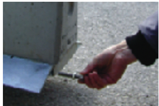
Insertion of the clamping bolts during the unloading procedure
