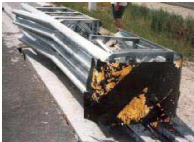
Damaged TRACC in Boise, Idaho
