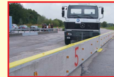
Tested safety: successful impact tests pursuant to DIN EN 1317 with trucks and cars at TÜV Süd in Munich.
