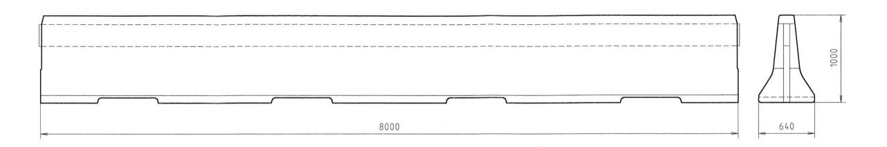
Note: the element is connected by the integrated coupling, located at the face of the element.
