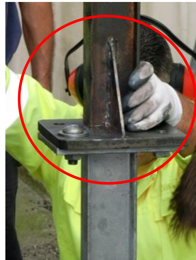
Fig. 10: Tool for the post driver screwed onto the post
