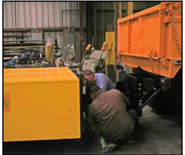
Figure 10. Bolt the TMA to the Support Bracket.
