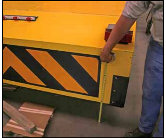
Figure 15. Adjust the level of the cartridge.
