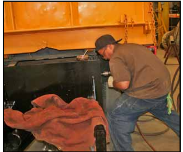
Figure 5. Drill holes through the frame rails.
