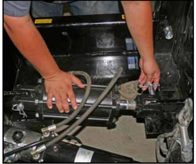
Figure 12. Install the lift cylinder.
