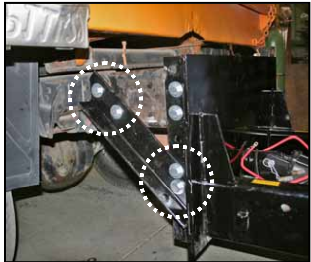
Figure 8. Bolt the side Channel Braces.
