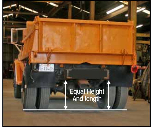
Figure 1. Frame rails are equal Height and length.
