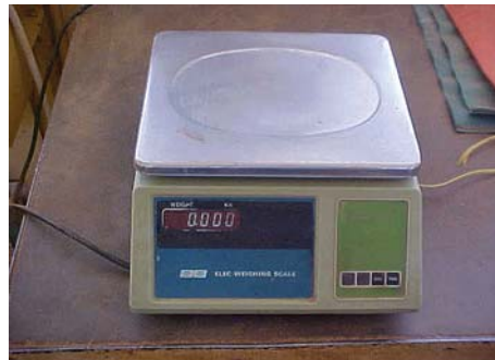
Figure 3.3: Sensitive balance on thick slate base to minimize vibrations.
