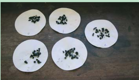
Bitumen Adhesion Test at ABCC unit.
