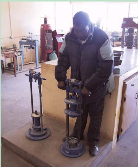
AIV test is also carried out at CML.
