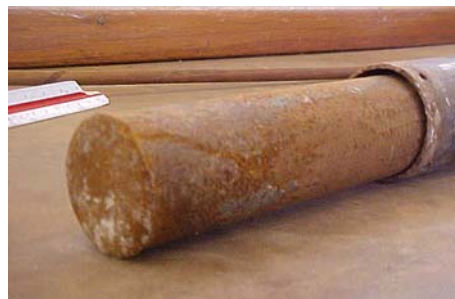
Figure 3.4: Worn compaction hammer with rounded face.
