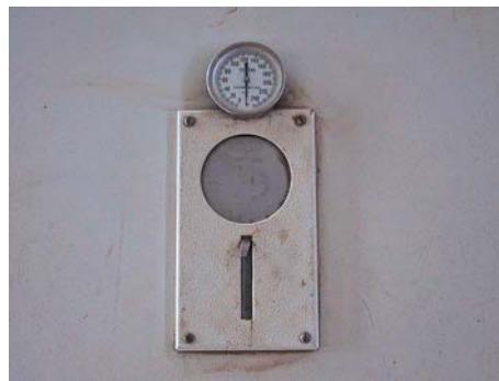
Figure 3.7: Thermometer positioned through hole on top of oven to check oven temperature directly.
