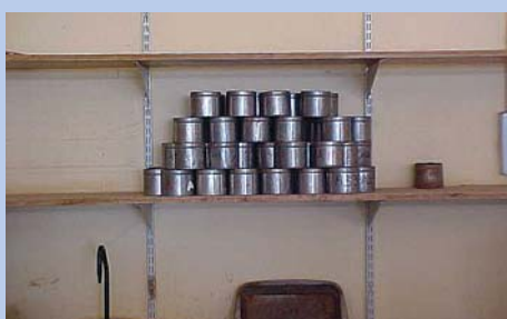
Special care must be taken of moisture content tins to avoid rust.
