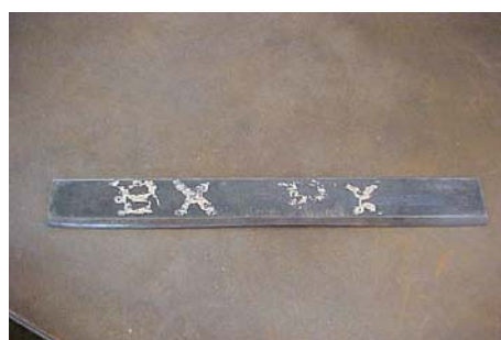
Figure 3.5: Straight edge that is no longer straight.
