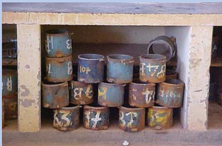
Compaction moulds like other equipments in the laboratory must be taken care of. Appropriate storage is imperative.
