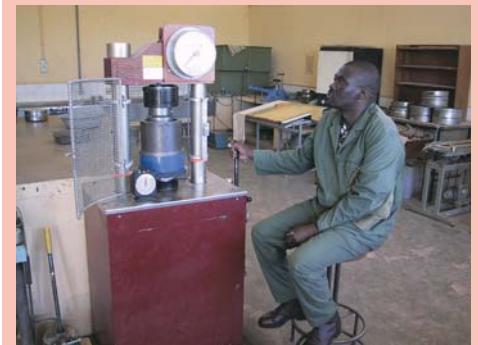
Compression machine shall not be operated while the safety cage is open.
