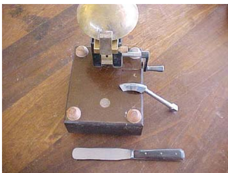
Figure 3.6: Indentation on the rubber base of the Atterberg Liquid Limit device caused by the fall of the cup and a worn out spatula. Such deformed equipment should be removed from the laboratory.
