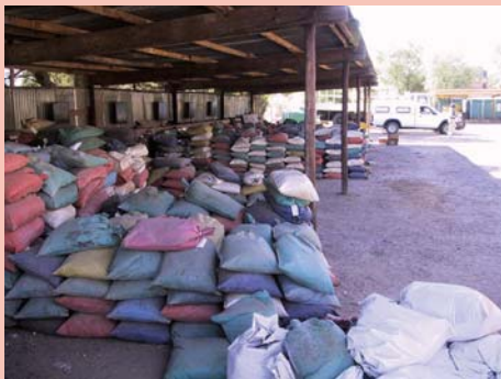
Samples shall be stored in a dry and clean environment in an orderly manner.
