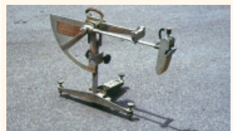
Pendulum tester to determine skid resistance.
