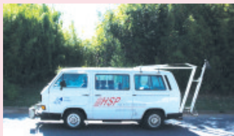
HSP showing rut measurement equipment at rear.
