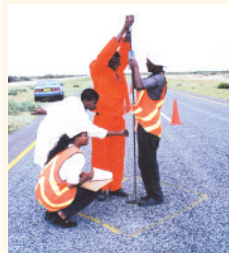
DCP testing, a useful tool in pavement evaluation.
