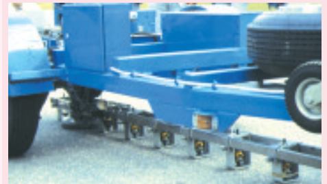
Falling Weight Deflectometer showing geophones.
