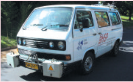
HSP showing laser based riding quality measurement apparatus.
