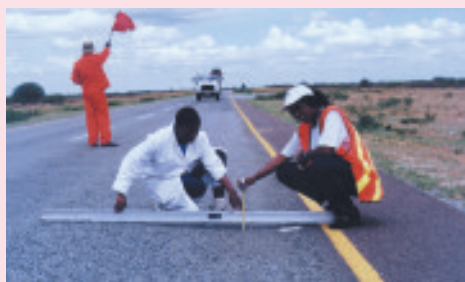
A rut measurement team in action. Note the flag man for safety reasons.
