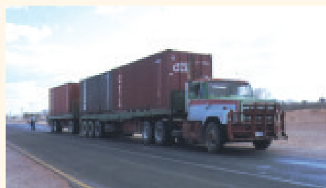
Overloaded vehicles are a major cause of premature distress due to the exponential effect of load on pavement damage. Hence the pavement life can be significantly reduced.
