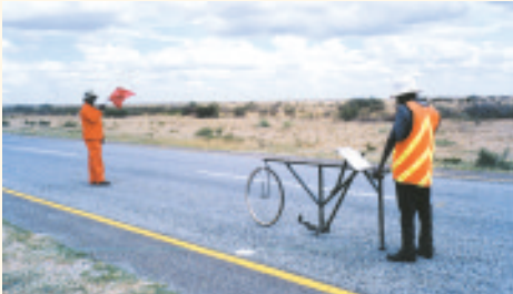
Measurements of roughness using a MERLIN apparatus.
