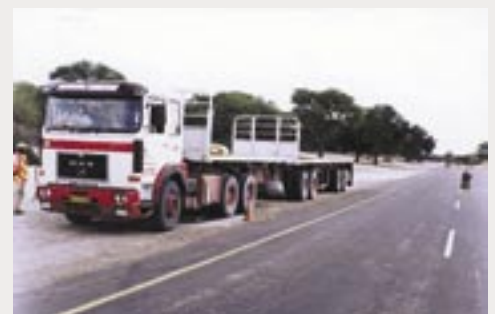
Empty trucks shall always be included in the axle load surveys, otherwise the VEF figures will be wrong and inaccurate.
