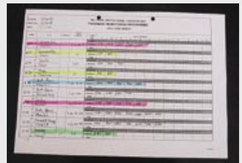
After entering that particular axle configuration it is important to mark the entered data with a highlighter. This to ensure that the data that has been entered are not being entered for the second time.
