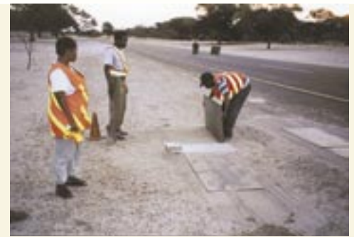
The mobile weigh bridges must be repositioned regularly to maintain correct readings.
