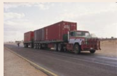
Heavy trucks and in particular those which are overloaded contribute significantly to the damage of the pavement, thus giving a shorter pavement life than designed for.
