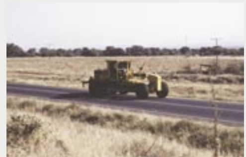
Specialised plant equipment i.e. a grader shall NOT be included in the axle load survey.
