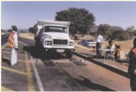
A correct selected weighing place with the scales correctly positioned.
