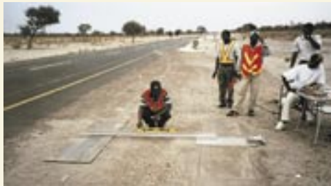
Correct cross wise gradient is a must for collecting data. The use of a spirit level and a straight edge.
