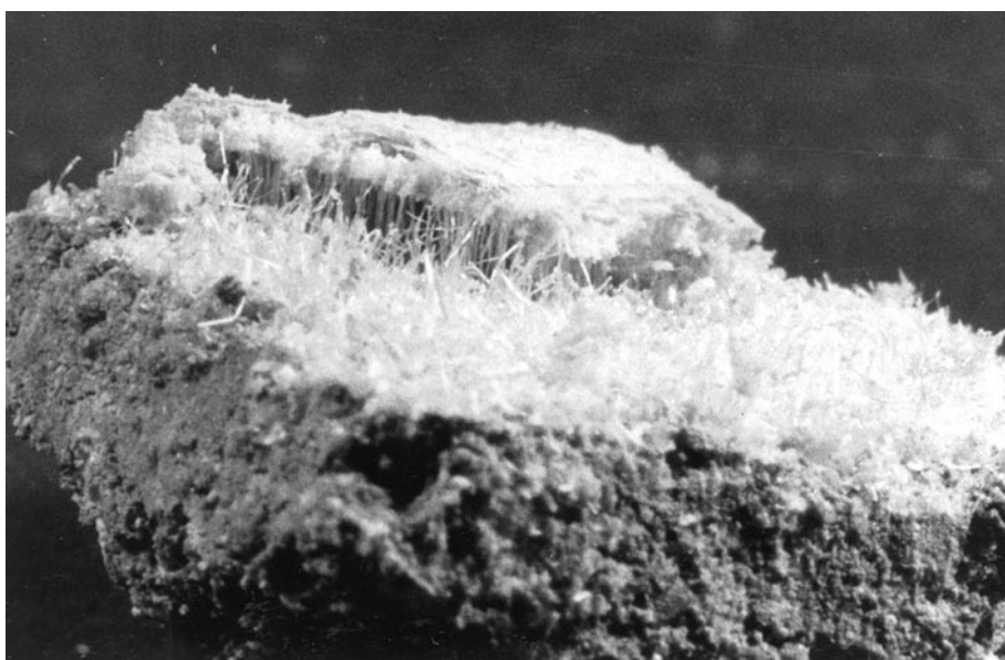
Whisker NaCl crystals cause maximum damage.
