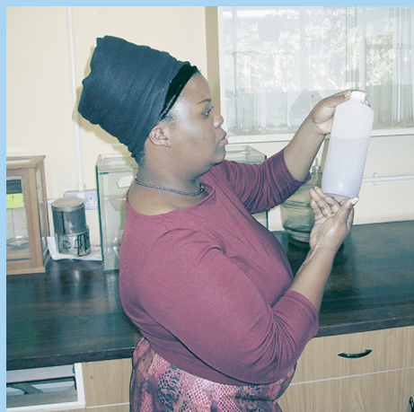
Water samples should be taken from near the surface of water sources to be used for construction.
