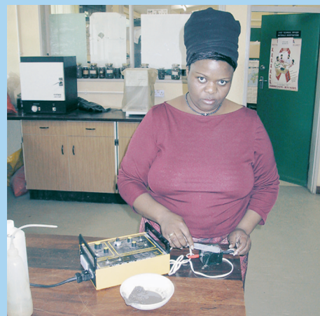
Electrical conductivity test carried out at the CML.
