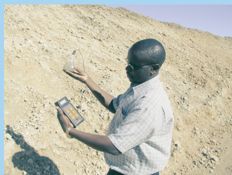
Hand held conductivity metre, is an accurate and quick method to measure salt content.
