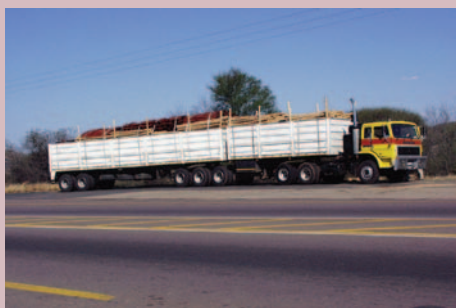
Load distribution over the various vehicle axle configurations determines the vertical load on the road.
