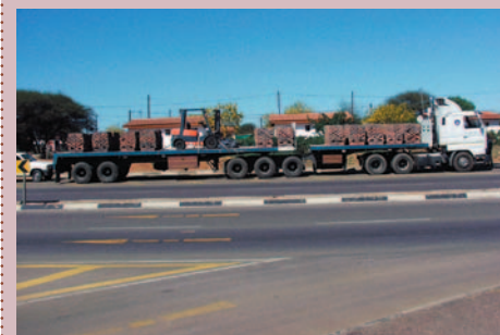
Vehicle classification can be determined by the number of axles and the gross vehicle mass.
