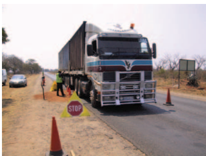
Axle load survey in progress. Such surveys are typically carried out over a 24 hour period for seven days.
