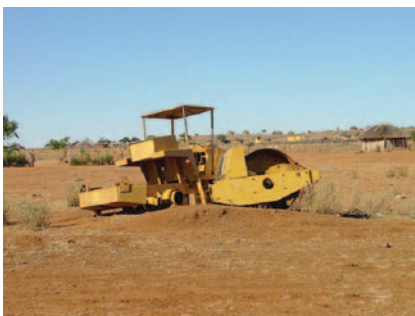
Very often, worn out construction plant is abandoned and becomes an eyesore. The contract documents should cover removal of unwanted plant to an approved area.
