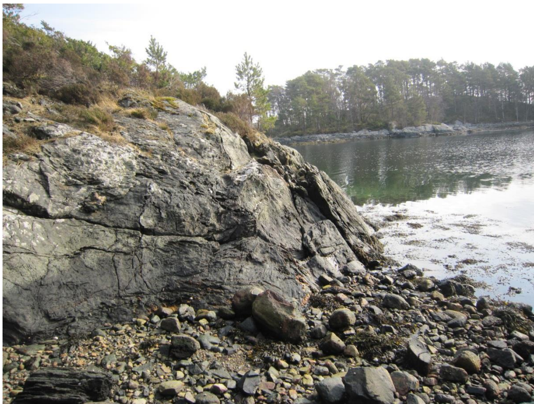
Figure 11 - Location 7, rock mass with irregular structure and jointing
