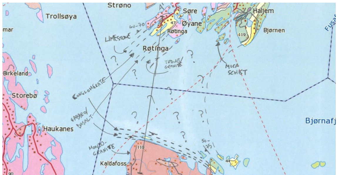
> Figure 4 Anticipated seabed geology, interpreted along the strait crossing.
