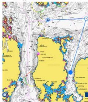
Figure 5-8 Towing from assembly site and turning of 4400 m end anchored bridge
