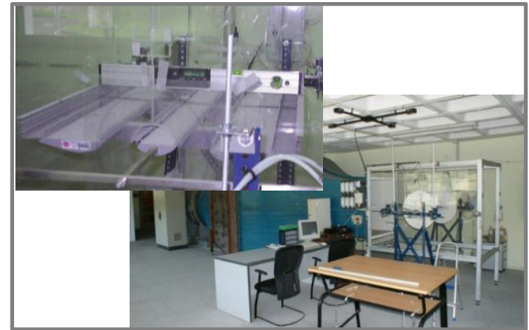
*Messina bridge sectional model, U. of Coruna
