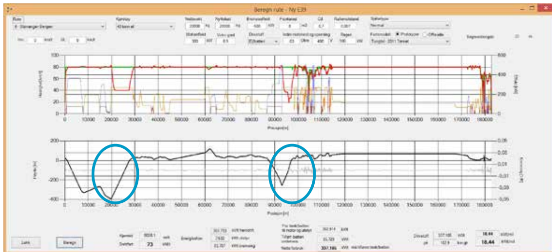
Blue circle: Direct use of the energy up two tunnel ascents can reduce the required battery capacity by a third.
